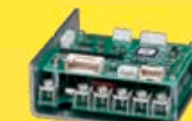
Dedicated driver for Nissei Corporation's battery-powered BLDC gearmotor
